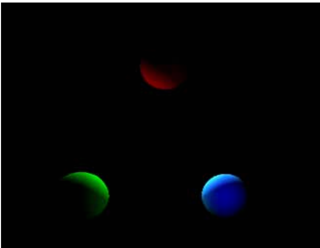
Output of deferred renderer's second pass that combines all G-buffer elements
