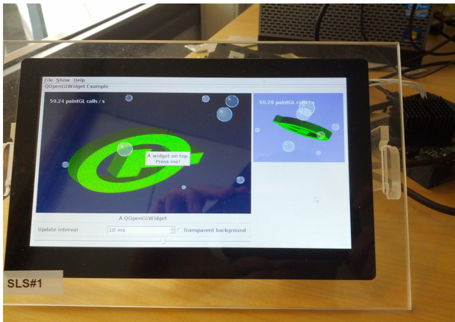
A QWidget with two QOpenGLWidgets running on i.MX6 Sabre LITE on eglfs
